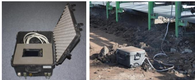
Fig. 3. View of open measuring system box with visible tablet and wiring and during its operation at belt conveyor.
