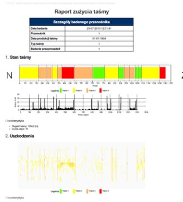
Fig. 7. Report showing belt condition visualization and damage histograms.
