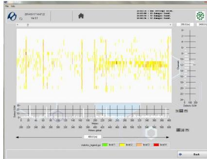
Fig. 6. Statistical analysis window with damage matrix and vertical and horizontal histograms.
